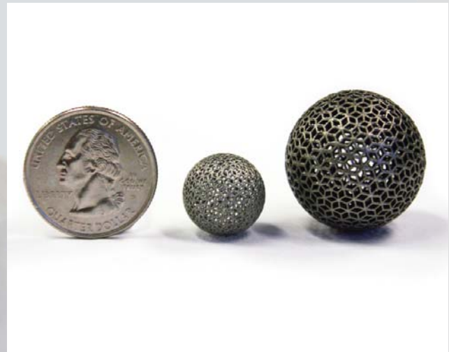
DMLS technology provides freedom of design while accurately reproducing fine feature details.
