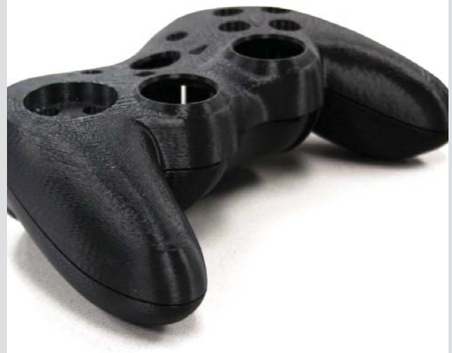
FDM ABS Black material was used to test the new design of this videogame control.
