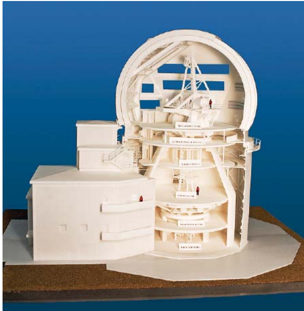
The completed architectural model consisted of 12 assembled SLS parts. Key pieces could be removed to expose internal areas.
