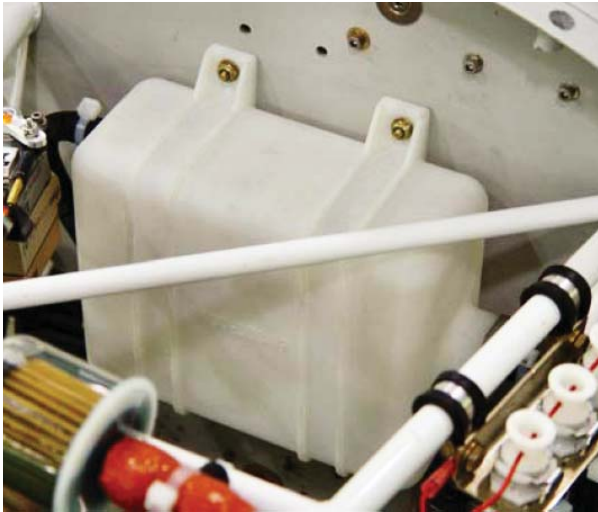
The new designed-for-SLS tank featured above integrates mounting brackets and support structures. The newly designed SLS tanks help provide longer flight times due to their light weight and increased fuel storage capabilities.
