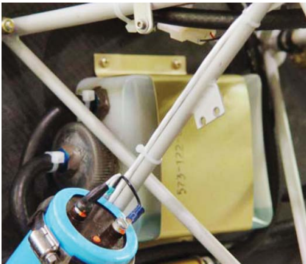
Pictured above is the original UAV Fuel Tank design complete with fastening hardware. The new SLS fuel tank design eliminated as many as seven piece parts and improved performance reliability.
